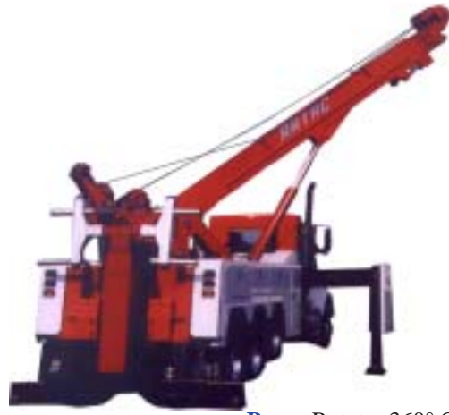
Boom Rotates 360° Continuously
